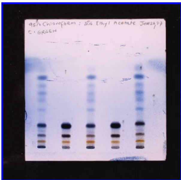
Figure 7. Ammonium molybdate/H 2 SO 4 spray reagent, white light.
