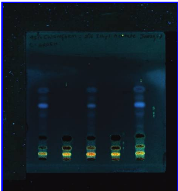
Figure 6. Ammonium molybdate/H 2 SO 4 spray reagent, 366 nm.
